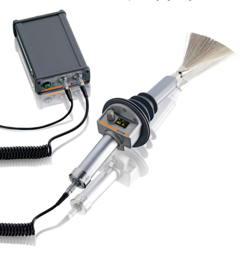
In order to protect objects, which are made of steel or metal, they are coated with corrosion resistant materials such as rubber, synthetics or enamel. The protective coatings must be tight, that is, free of pores, cracks or embedded foreign objects, to keep aggressive materials from the carrier material that is in danger of corrosion. Fine pores or cracks cannot be entirely avoided in any coating process.
