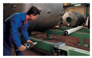
Testing the interior coating of a pipe with the POROSCOPE®, using a rotating electrode on a rod extension system
