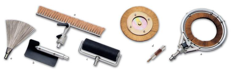
Overview of the various electrodes: a) Sweeper electrode b) Flat electrode c) Roller electrode d) Rotating electrodes for tests inside pipes e) Circular ring electrode for tests on the outside walls of pipes
