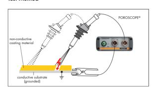
The test method is based on the fact that all electrically insulating coating materials have a much higher disruptive strength than air.
