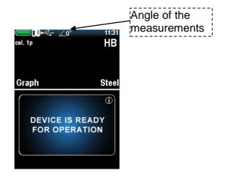
Position of the probe perpendicular to the ground plane corresponds to the angle  $0^{\circ}$ .
