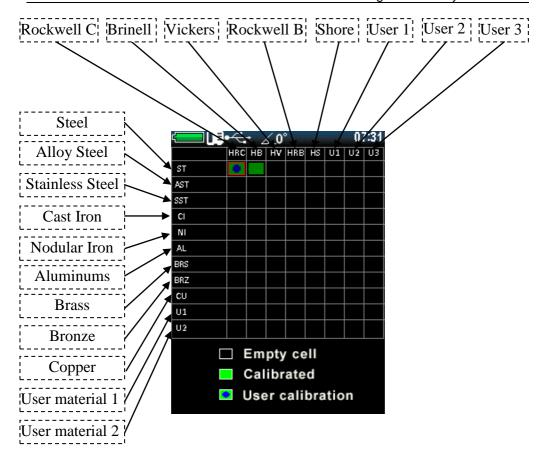
Each of the scales can be calibrated to 11 conventional materials: Steel (ST), Alloy Steel (AST), Stainless steel (SST), Cast Iron (CI), Nodular Iron (NI), Aluminums (AI), Brass (BRS), Bronze (BRZ), Copper (CU), User material 1 (U1), User material 2 (U2).
