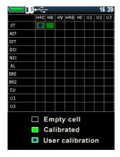
To delete user calibration, go to the user calibration mode and set to **0** for **N**:
