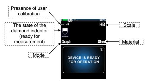
Then select the scale and material hardness for which there is a proper calibration (how to calibrate device see paragraph 11).
