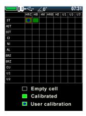
Each of the scales can be additionally calibrated by 1 or 2 points. Also, the unit measures in Leeb scale (with rebound probe) and Tensile strength, through the automatic recalculation of the Brinell scale.
