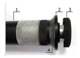
Figure 1a. UCI Probe U1 1 – Probe's body; 2 – Collapsible nozzle; 3 – Puck; 4 – Place for fingers
