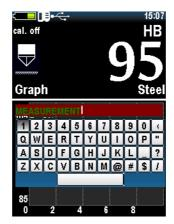
Move the cursor over the keyboard with navigation keys and select symbols by pressing . Then press for saving. The record is stored in the archive.
