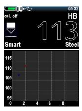
Filled with the color readings indicate that the device has fixed the general sequence and Smart mode is active.
