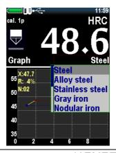
During the measurement you can select other hardness scale. The displayed measurement reading will be converted according with the new hardness scale if it is calibrated.
