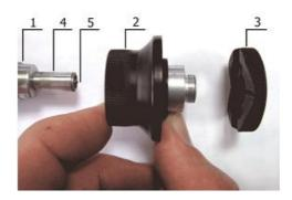
Figure 1b. Demounted nozzle
