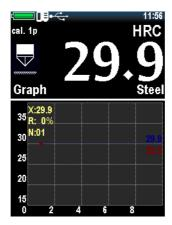
In graph mode, the device displays the current measurement value or average of series of measurements, depending on selected the Current or Average in Measurement settings menu:
