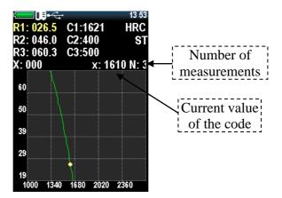
If you get an obvious error measurement, press and the last measurement will be removed from the series.
