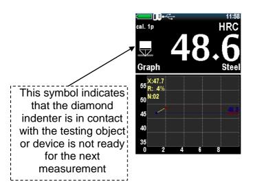
WARNING! Not allowed a sharp click and scratching sample by indenter, this may lead to exceeding the allowable value of error and damage the diamond indenter.
