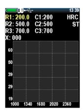
The device, making the measurement, gets the nominal codes, the purpose of calibration - is to find the correlation between the nominal code and hardness values (construction of the relation function).
