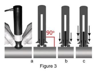
NOTE! For correct operation of the UCI probe try not to exceed the pressing force which is correspond to the probe (1 or 5 kg).
