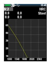
Move the cursor by pressing to select the first row. Take about 5 measurements on the first sample, the instrument will display the average of the series in accordance with the current
