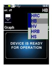
For select the material press and chose the material that will be used by keys and then press .
