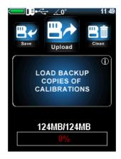
After the initial save of calibrations you can always download it to the probe. This function is needed for the resumption of adequate calibration in case of wrong settings of the probe.
