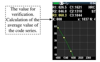
To check the correctness of the got values, move the cursor to the **X:000** and take a few measurements on one of the sample.
