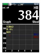
WARNING! The minimum distance between the imprints of measurements must be not less than 3 mm.
