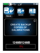
After calibration of the probe is recommended to create a backup copy of the calibration (usually the manufacturer makes the calibration of 1-2 scales, to check the probe). This is done in order to be able to resume adequate calibration after incorrect settings in the future.
