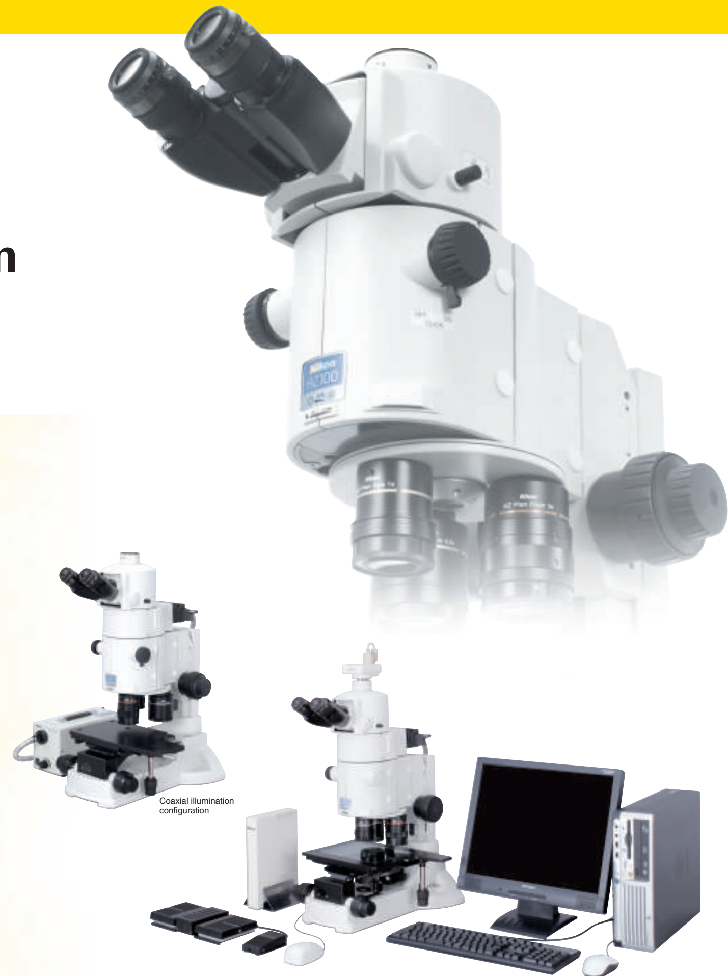
Coaxial illumination configuration + digital camera DS-F1 + controller accessories
