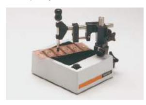
**Angle probe Z11NG in the support stand V12** For coating thickness measurement in sleeves, pipes, bearing shells etc. of 32 mm diameter and more.
