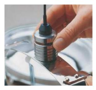
Probe for inside diameters Z3NG for measurement in holes. Touchdown probe Z3NG-A for measurement on very small measuring surfaces.
