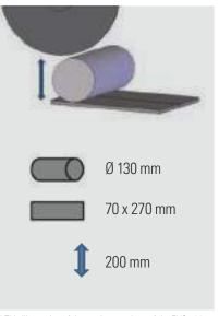
\* This illustration of the cutting envelope of the EVO 400 is to show the maximum theoretical capacity only. The actual capacity in practice will depend on the sample geometry and its physical properties.
