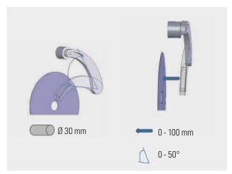
\* This illustration of the cutting envelope of the MECATOME T330 is to show the maximum theoretical capacity only. The actual capacity in practice will depend on the sample geometry and its physical properties.
