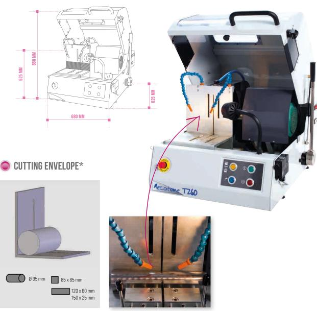
\* This illustration of the cutting envelope of the MECATOME T260 is to show the maximum theoretical capacity only. The actual capacity in practice will depend on the sample geometry and its physical properties.
