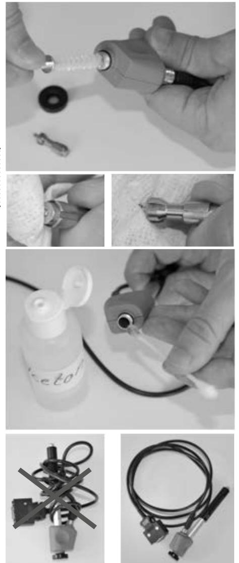
Figure 9: Maintenance and cleaning procedures
