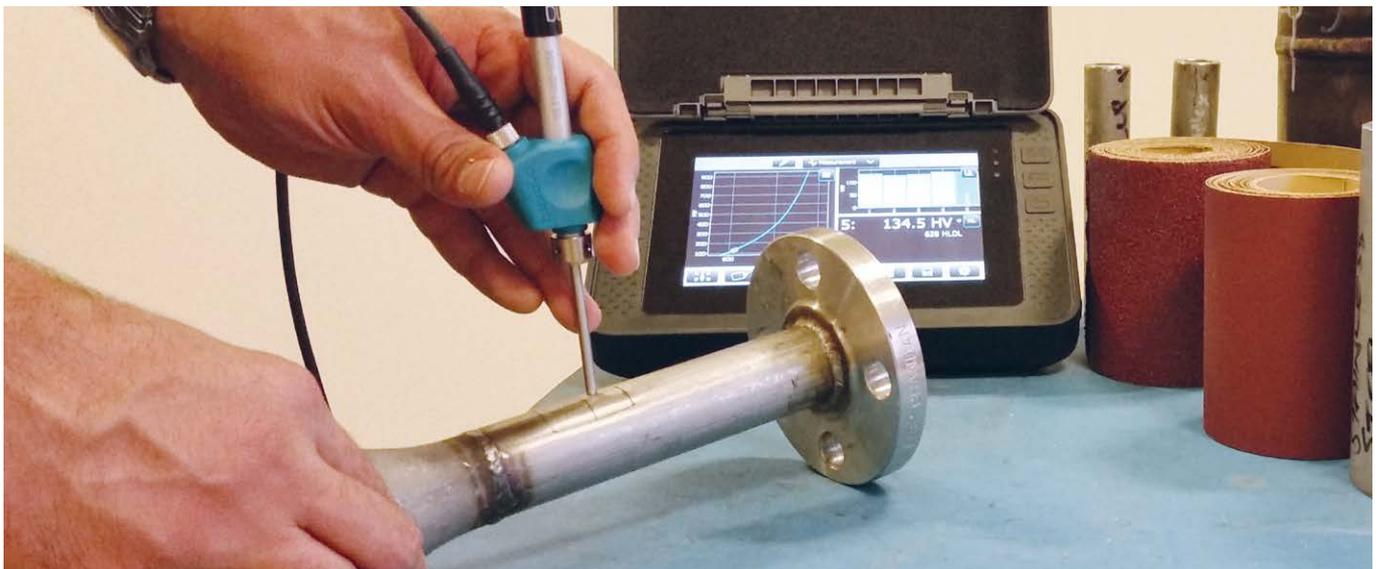
Figure 26: Performing Leeb measurements on test sample
