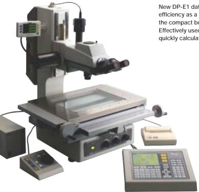
New DP-E1 data processor has been developed to improve accuracy and efficiency as a measuring system. A 0.1 $\mu$ m-reading counter display is built into the compact body. The 320 x 240-pixel LCD greatly improves ease of use. Effectively used in combination with a measuring microscope/profile projector, it quickly calculates and processes measurement data.
