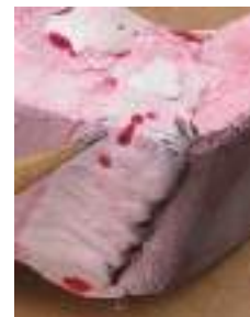
Fluorescent penetrant indications using Method C
