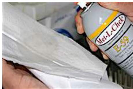
Apply E-59 to cloth to wipe remove surface penetrant.
