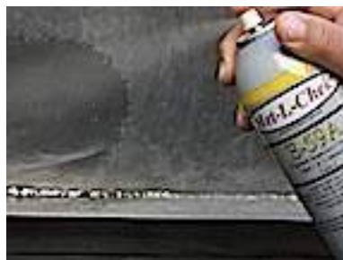
E-59A used as a pre-cleaner spray directly on test surface and wipe clean.
