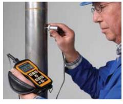
DM5E ultrasonic thickness gaging of pipes
