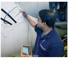
Aircraft inspection with the Phasec 3 series flaw detectors
