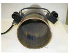
Eddy current surface and subsurface inspection for flaw detection in metals
