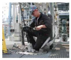
Inspecting chemical plant vessel with Ca-Zoom® PTZ inspection system
