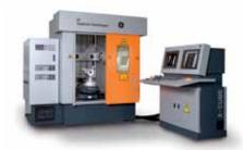
X-cube  $^{\textcircled{R}}$  is a highly versatile 160/225 KV inspection system.
