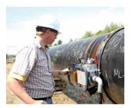
Weldstar mobile ultrasonic inspection system
