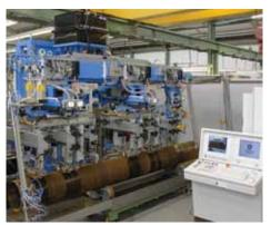
SNUP ultrasonic pipe testing system
