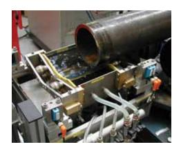
$\ensuremath{\mathsf{GRP}}$  ultrasonic tube and pipe testing system
