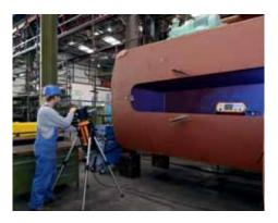
Inspection of ship assemblies using industrial X-ray
