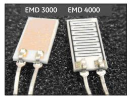
Figure 1: EMD3000 and EMD 4000 Sensors
