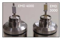
Figure 2: EMD3000 and EMD 4000 Sensors on Loggers
