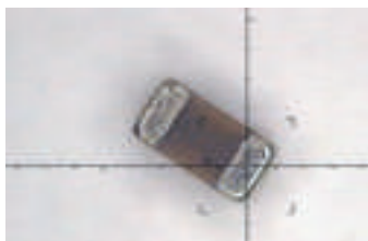
SMD component: Checking for lead content
