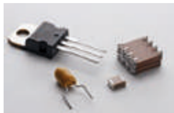
High reliability: Pb (> 3 %) in electronic components
