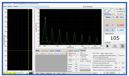
According to API-653, specifications of the storage tanks can be included, to calculate minimum acceptable thickness and maximum allowable tank capacity.
